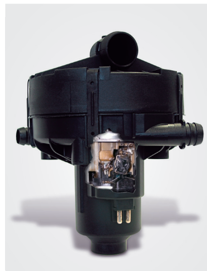
View into the secondary air pump (cut) with melting traces
