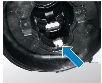
Damage symptoms: Melting traces on the housing (top view into the housing)
