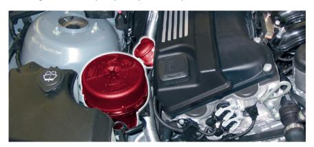
Secondary air valve and secondary air pump in BMW E46 (highlighted)
