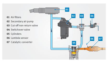
Block diagram of secondary air system (pneumatically actuated)
