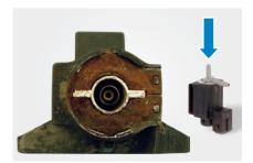
Corroded switchover valve (open)
