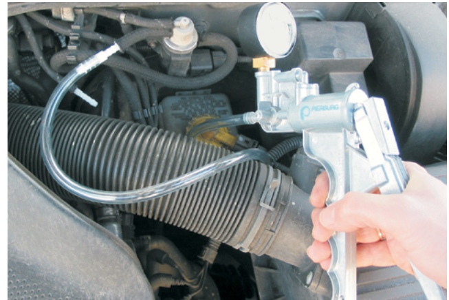
Checking a pressure transducer using a manually operated vacuum pump (VW Golf IV) (Pierburg Art. Nr. 12 00001 11 900)
