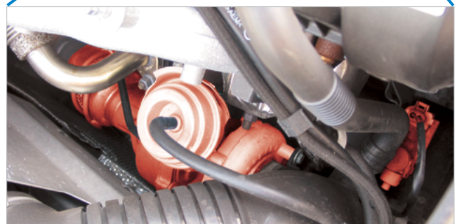
Pressure transducer and VTG charger (highlighted in red) in the Audi A4 TDI
